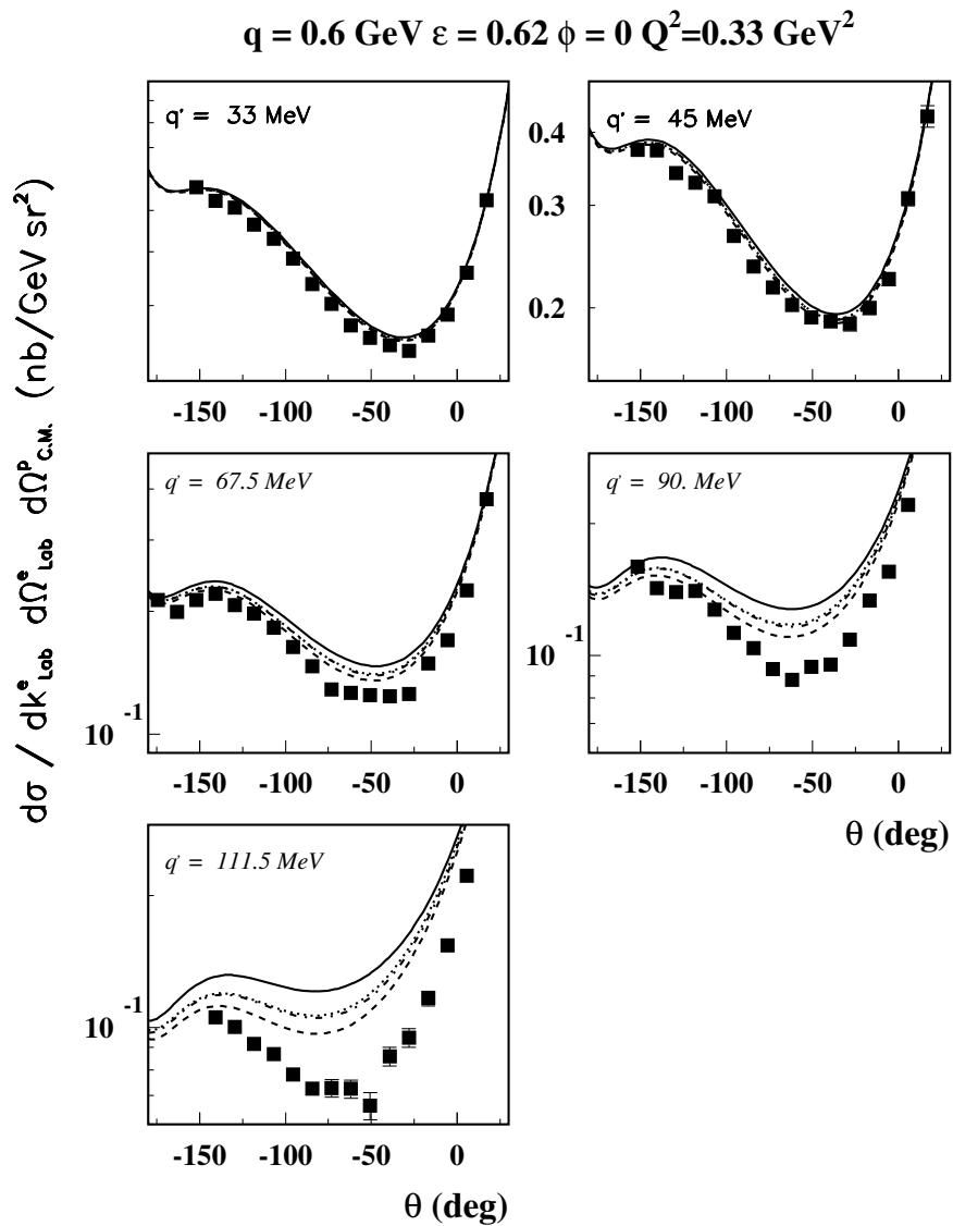
**Differential cross section for  $ep \rightarrow ep\gamma$  as function of the photon scattering angle in the MAMI kinematics specified in the plot.<sup>a</sup>**
