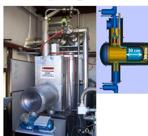
20L vessel of liquid parahydrogen
